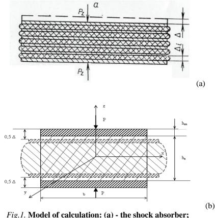
Fig.1. Model of calculation: (a) - the shock absorber; (b)  $- n^{th}$  - layer of shock absorber
