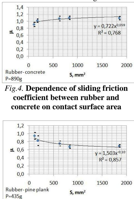
Fig. 4. Dependence of sliding friction coefficient between rubber and concrete on contact surface area
