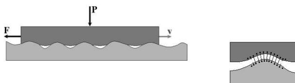
Fig.8. Interdependent positioning of sliding surfaces and bonds between their atoms
