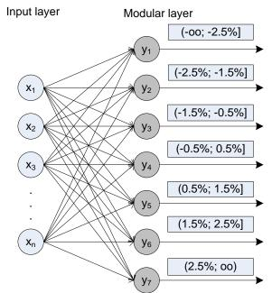
Fig. 11. Modular neural network for interval value prediction
