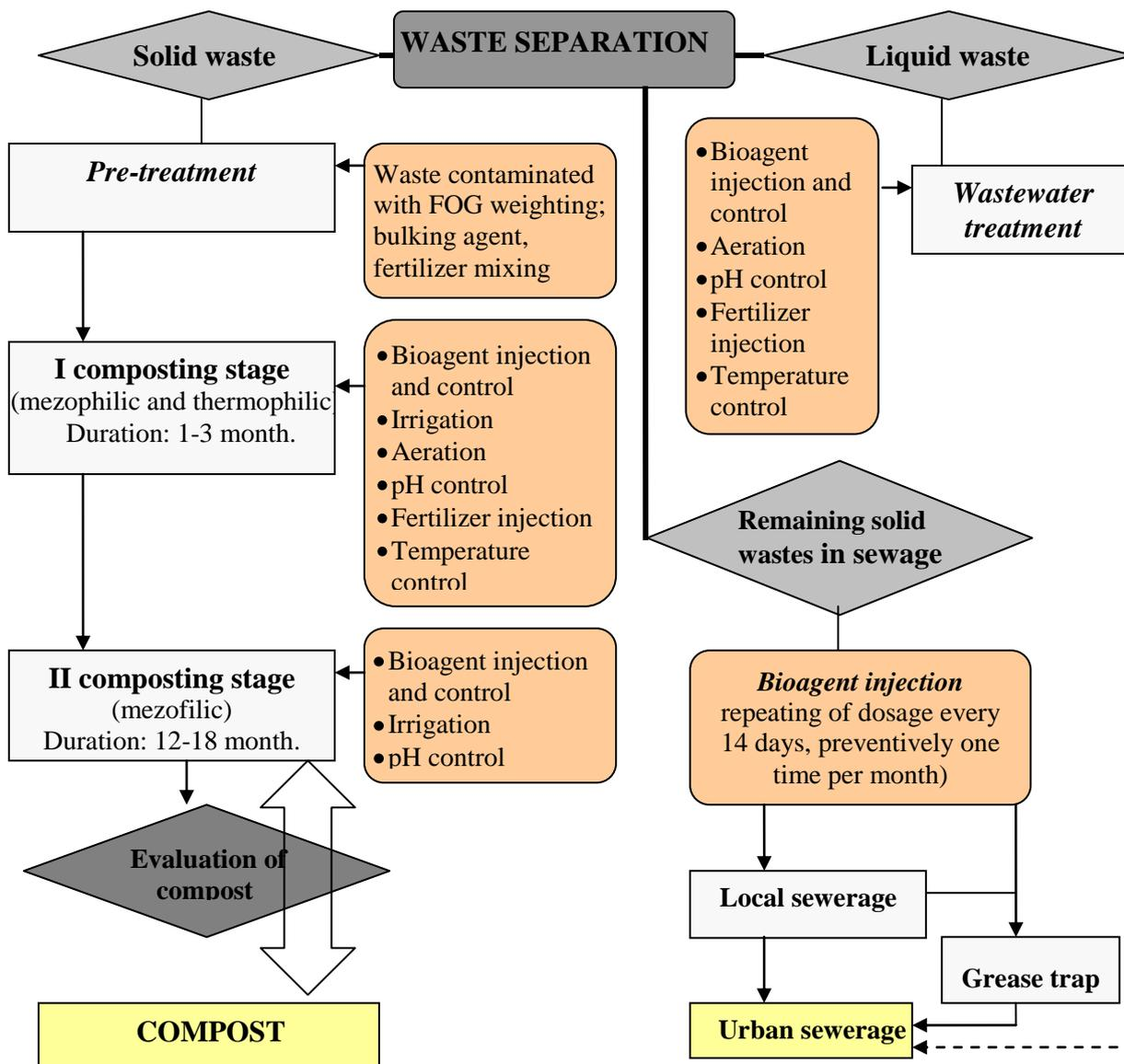
Fig.1. Complex technological for grease wastes utilization diagram
