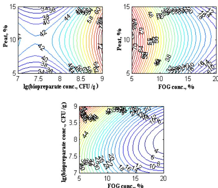
**Fig.4. Dependence of the degraded fat percentage (after 2 weeks) on the technological parameters: percentage of fat, inoculate cell concentration of bacterial composition and the percentage of peat in the vicinity of maximum degraded fat percentage point.**
