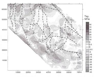
Fig. 7. SDS simulation,  $\tau_{xy}$  component
