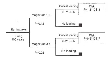
Fig. 4. Event tree for earthquake during 100 years
