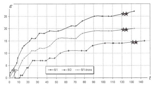
Fig.1. Roof-to-floor convergence curves
