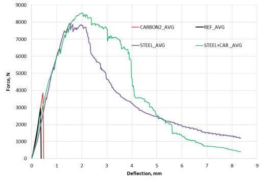
Fig. 3. Three-point bending force – deflection curves.
