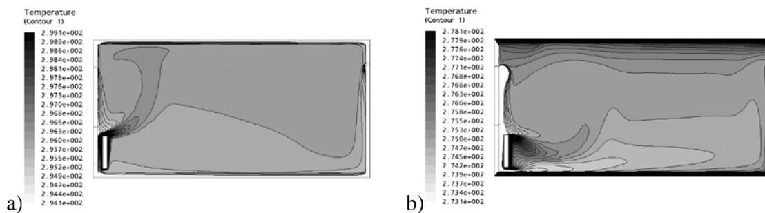
Fig. 6. Temperature distribution in a room in variants 2-1 (a) and 2-2 (b)
