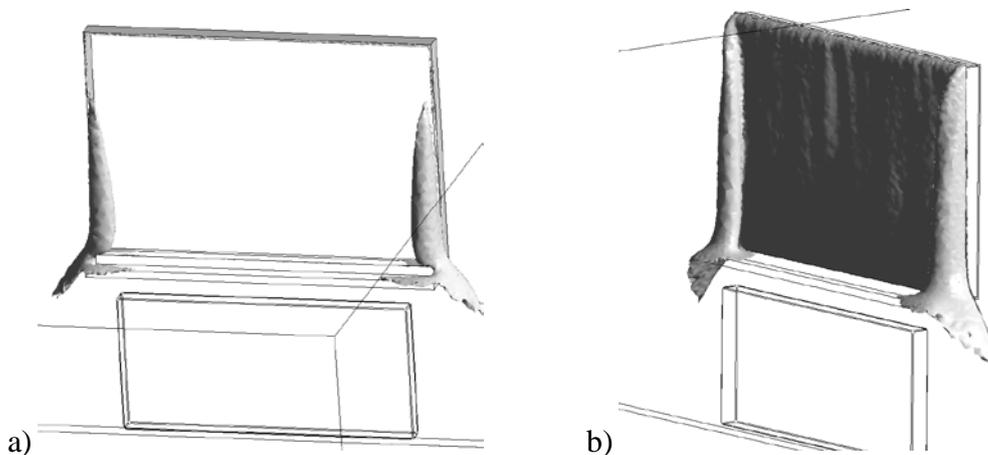
Fig. 8. Isosurfaces of  $v=0,55 \text{ m/s}$  (a) and  $T=7^\circ\text{C}$  (b) for modelling variant 3-1
