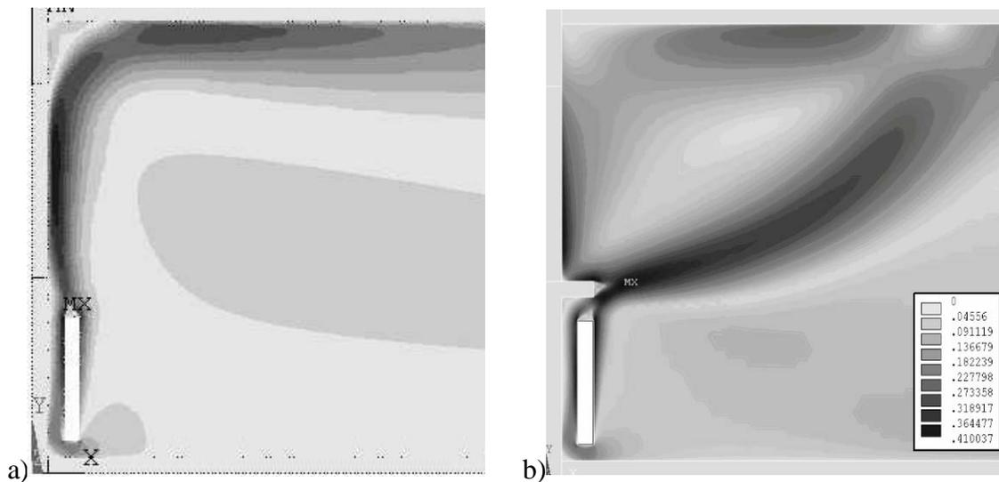
**Fig. 3. Stationary distribution of the velocity modulus in the modelled room.**
