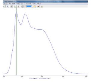
Fig. 6. Lamp's spectral characteristic. The current through the blue and green LEDs is 350mA; through Samsung LED module 300mA.
