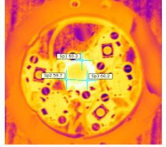
Fig. 15. Second regime of operation. IR photo of LED lamp. Sp – measured solder point temperatures. Ambient temperature Ta=42°C  $\,$
