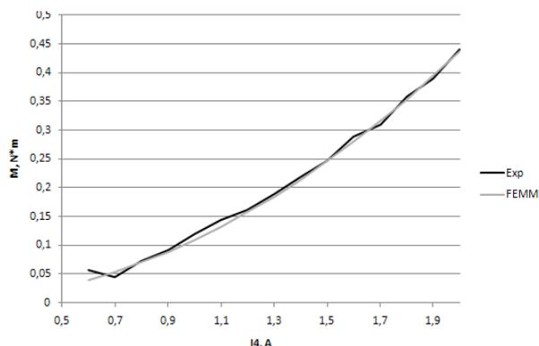
Fig. 6. Torque depending on the drive windings currents.
