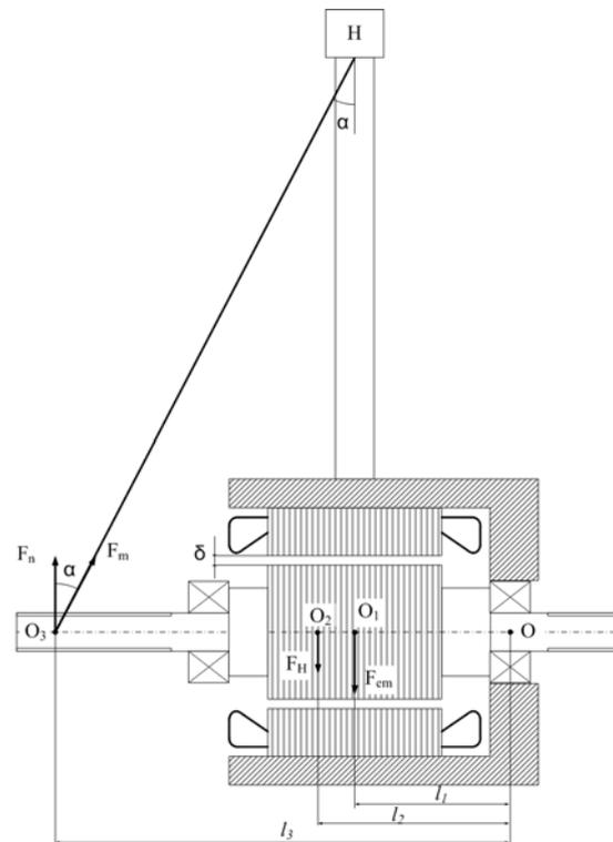
Fig. 4. Scheme for radial forces research .
