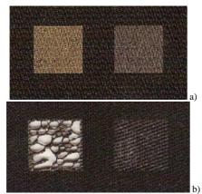
Fig. 9. Laser treating by: a) carbonation; b) melting.
