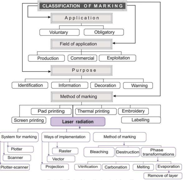
Fig. 15. Classification of the markings by various indicators [3]
