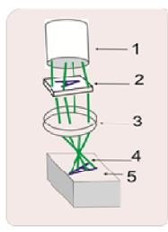
Fig. 3. Projection Marking where: 1-laser, 2-mask, 3-lens, 4-image, 5-work area [3].
