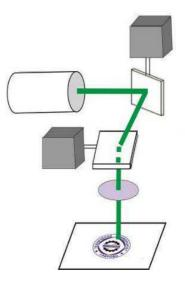
Fig. 5. Scanner system for marking [3].
