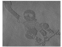
Fig. 10. Laser treating by evaporation (ablation) on polar fabric.
