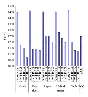
Fig. 2. Initial melting temperature (ST) of different energy crops and their mixtures: w- the particular species of wood, RCG – reed canary grass
