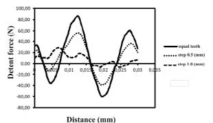
Fig.10. Detent force relation to step size 0.5 and 1 mm, for decreasing the teeth length
