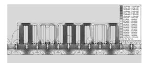
Fig. 3. The motor magnetic field distribution in final loop step
