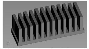
Fig.7. Mover ferromagnetic core with teeth with progressively decrease
