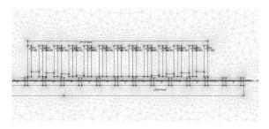
Fig.8. FEM model of the linear motor with a mover ferromagnetic core with teeth of different lengths
