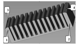
Fig.4. 3D CAD model of mover core
