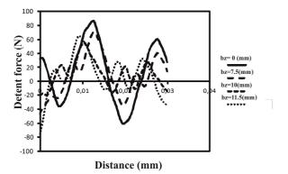
Fig.6. Detent force in relation to the additional teeth width
