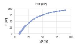
Fig. 7. Mapping of values of power regulation coefficient kP [%] to CO2 laser power P [W].
