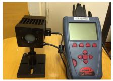
Fig. 8. Power measurement sensor OPHIR F150A-BB-26
