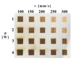
Fig. 12. Outcomes after CO2 laser treatment on white color artificial leather material.
