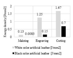
Fig. 20. Values of energy density required for marking, engraving and cutting of black and white color artificial leather using CO<sub>2</sub> laser plotted in chart.
