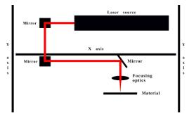
Fig. 6. Schematic view of experimental set-up of SUNTOP ST-CC9060 CO, laser system.
