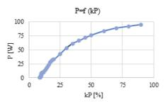
Fig. 5. Mapping of values of power regulation coefficient kP [%] to fiber laser power P [W] with a constant pulse repetition frequency f = 30 [kHz].
