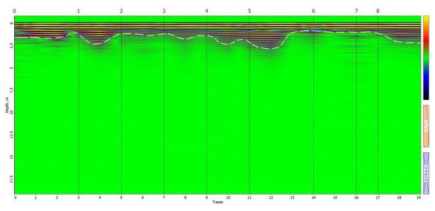
Fig. 4. Radargram showing GPR profile obtained by geophysical survey with 75 MHz antennae from the ice surface
