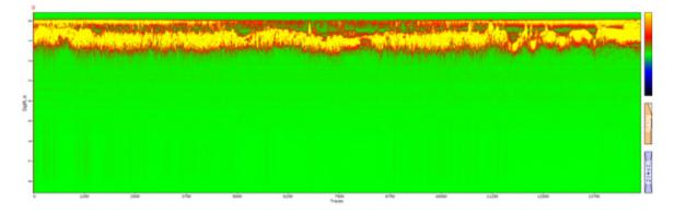
Fig. 7. Processed GPR profile obtained by geophysical survey with 500 MHz antennae from the inflatable boat along the transect No.2 in lake Zeilu
