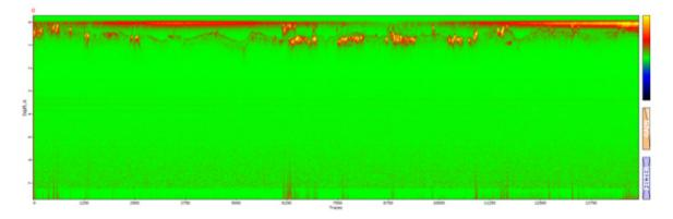
Fig. 9. Processed GPR profile obtained by geophysical survey with 500 MHz antennae from the inflatable boat along the transect No.4 in lake Zeilu
