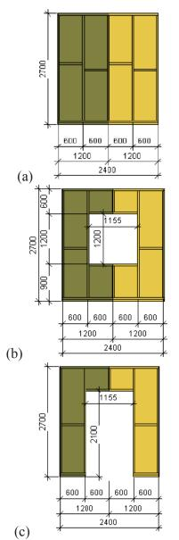
Fig. 8. Three variants of considered shear wall panels: a) – variant without opening; b) – variant with window opening; c) – variant with door opening [8].
