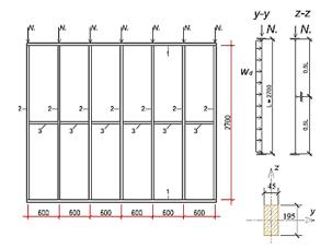
Fig. 7. Design scheme of the struts in shear walls in planes y-y and z-z.1 – head binders; 2 – struts; 3 – cross-bars [8].
