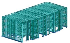
Fig. 6. 3D model of three-storey light framework's structures developed by software Autodesk Revit [8].
