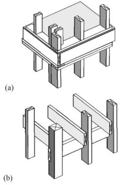
Fig. 3. Light framework's structural solutions: (a) platform framing; (b) balloon framing [8] – [9].
