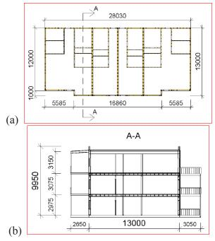
Fig. 4. Plan (a) and cross-section (b) of considered three-storey building [8].
