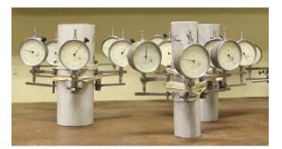
Fig. 3. Specimens prepared for shrinkage testing.
