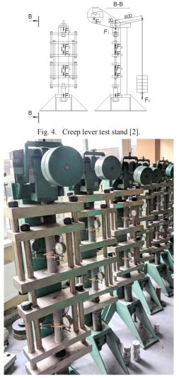
Fig. 5. Creep lever test stands with foamed concrete specimens inserted.
