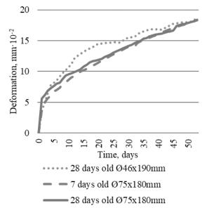
Fig. 6. Foamed concrete specimen total deformations.
