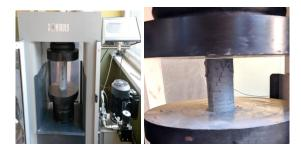
Fig. 1. Specimen compressive strength test.
