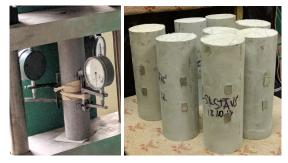
Fig. 2. Specimens prepared for creep testing.
