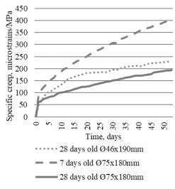
Fig. 7. Foamed concrete specimen specific creep.
