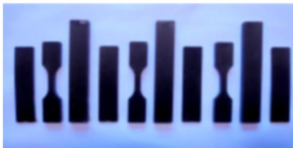
Fig. 5. Wood polymer composite samples obtained for testing
