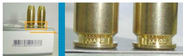
Fig. 1. Brass ammunition cartridge laser marking. [2]
