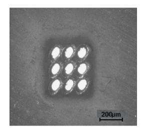
Fig. 10. Sieve on Stainless steel, thickness 150 $\mu$ m, scanning speed 50mm/s, number of repetitions - 20
