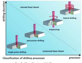
Fig. 3. Classification of drilling processes
