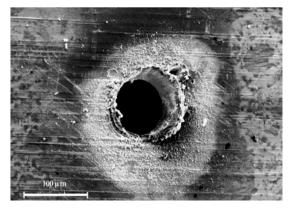
Fig. 8. SEM of the surface of Cupper foil, thickness 150µm, scanning speed - 20mm/s, number of repetitions – 2.
