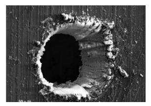
Fig. 7. SEM of the surface of Aluminium foil, thickness 100µm, scanning speed - 20mm/s, number of repetitions – 3.
