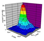
Fig. 2. Spatial distribution of power density at focal point of the laser beam after 1m focusing lens.
