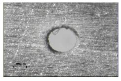
Fig. 5. Al foil, thickness  $100\mu m$ , scanning speed -20mm/s and number of repetitions -3.
