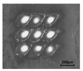
Fig. 9. Sieve on Stainless steel, thickness  $150\mu m$ , scanning speed  $150 \mu m/s$ , number of repetitions - 65
