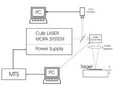
Fig. 1. Schematic of the experimental complex for laser micromachining.
