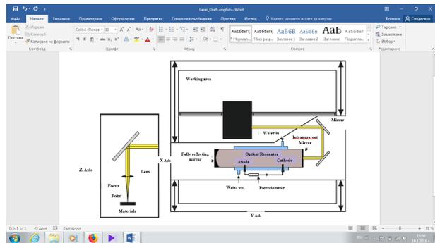
Fig. 3. Schematic diagram of CO<sub>2</sub> laser
