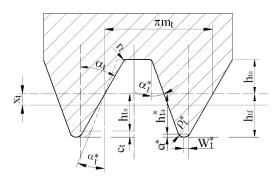
Fig. 3. Congruent output contour for possibility II of generation of asymmetric gear profile in the front section
