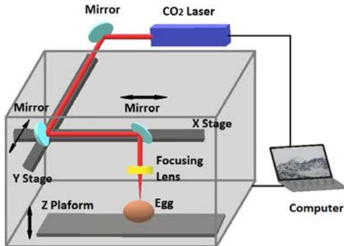
Figure 2a. Schematic diagram of an experimental setup for marking chicken eggs using a CO<sub>2</sub> laser.
