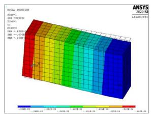
Fig. 6. Displacement in Y direction of the beam in ANSYS.
