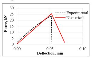
Fig. 7. Averaged experimental load bearing curve comparison with numerical simulation results for prisms without fibres (Group A).
