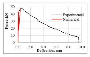
Fig. 8. Averaged experimental load bearing curve comparison with numerical simulation results for prisms with fibres (Group B).
