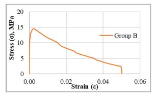
Fig. 3. 4PBT averaged experimental stress-strain curves of concrete for 28 days for Group B.
