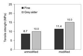
Fig. 1. Tensile strength of polymer composites filled with intial wood bark and modified ones
