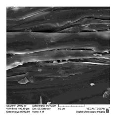
Fig. 5. Structural consolidation of filler particles in the composite, containing pine bark modified with DEEPA (50% recycled polyprolylene/50% modified pine bark)
