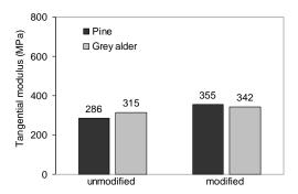
Fig. 4. Tangential modulus of polymer composites filled with intial wood bark and modified ones
