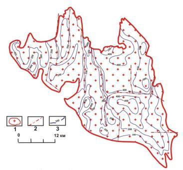
*Fig.3.* **Scheme of NKM top edge morphology** 1- NKM contour; 2- main faults; 3- contour lines of NKM top edge
