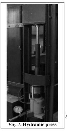
can be realized required force – displacement characteristic of compacting. Innovative press mechanism in shape of rhomboid linkage with hydraulic drive (Patent LV 14201) is recommended for briquetting of stalk material biomass.
