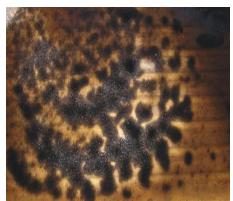
Fig. 4. Water surface after reaction with the ferromagnetic adsorbent
