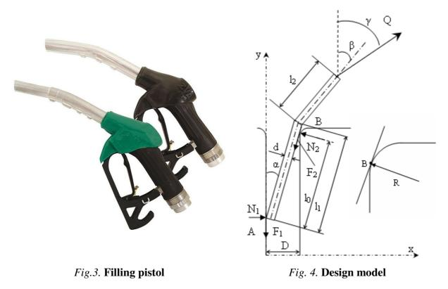
The reaction  $F_1$  and  $F_2$  directed opposite to the outer movement of the pistol. Let us write the equation describing the relationship of geometric dimensions:
