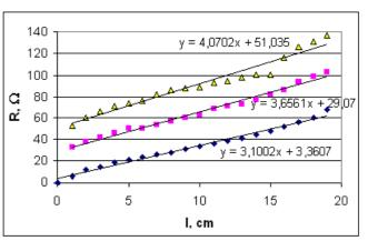
*Fig.11.* Electrical resistance of Al-Ti-N nano-coating deposited on the dielectric film (at frequency 1MHz) depending on the length of the section of the slip
