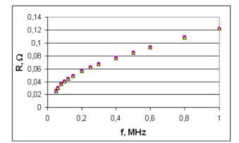
*Fig.5.* Curve of electrical resistance frequencies of the steel tube with leads and contacts
