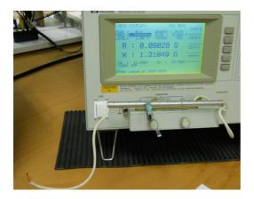
*Fig.6.* HP 4284A 20Hz- 1MHz LCR meter with the connected steel tube, resistance of the 10 cm long section is measured
