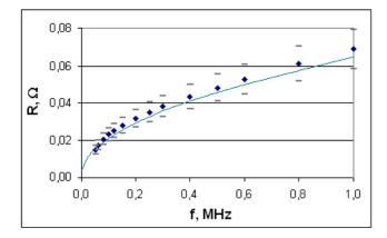
*Fig.8.* The curve of electrical resistance frequencies of the steel tube (without the leads and contacts)
