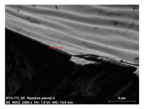
*Fig.13.* Fragment of the Al-Ti-N nanocoating that has separated from the surface of the dielectric film; its thickness is 523nm
