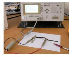
*Fig.10.* Measuring electrical resistance of Al-Ti-N nano-coating deposited on the dielectric film
