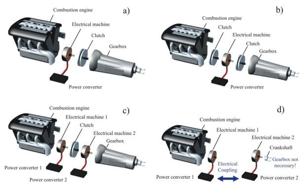
Fig. 1. Power train topologies for hybrid electric vehicles
