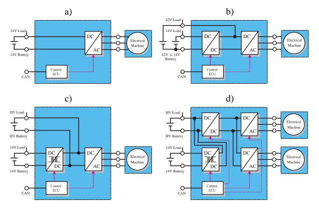
Fig. 2. Electrical system architectures for hybrid electric vehicles
