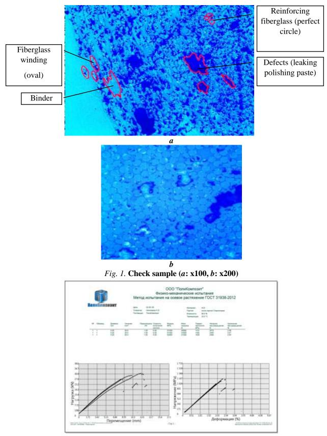
Fig. 2. The tensile strength of 1110 MPa, Modulus of elasticity 51733 MPa
