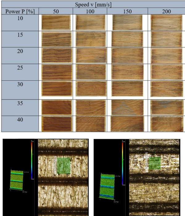
Fig.8. Measured result under a microscope with a magnification 5x to engraved plywood material with power P = 20 % and speed v = 200 mm/s. Line depth is 470  $\mu$ m.
