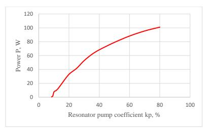
Fig.3 Dependence of the radiation power P on the resonator pump coefficient  $k_P$  %
