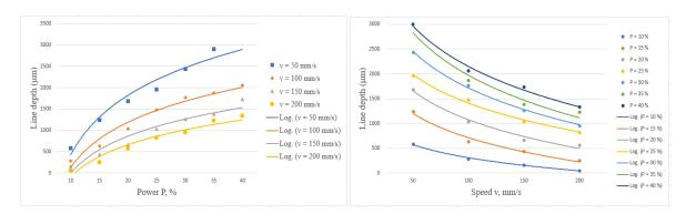
Fig.4. Graph of line depth values on plywood material depending as power change.
