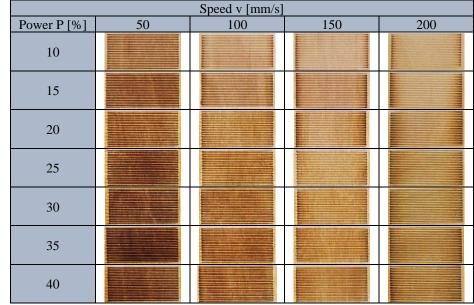
Table.1. Summary of data for marked and engraved lines of plywood series. Distance between marked and engraved lines  $\Delta x = 1$  mm.
