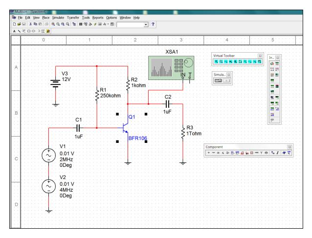
Figure 1 The example of UI in software
