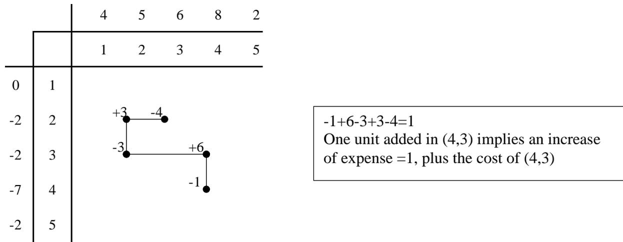
Figure 5 Increase in (4,3) using the closed path (3a)
