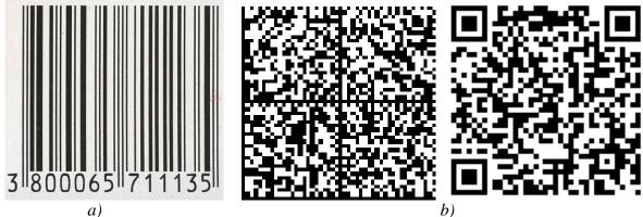
Figure 2 Marking of barcodes: a) 1D; b) 2D. (Sources: Pontius, 2012; Adams, 2014)
