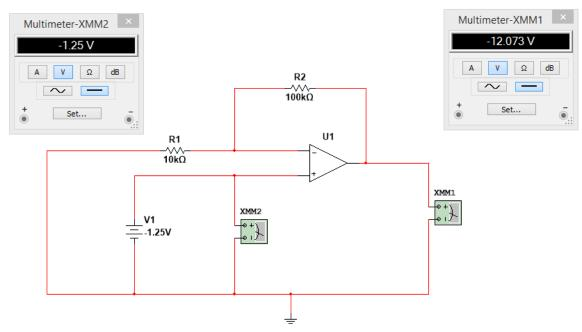
Figure 2 Diagram presenting the first circuit for testing a MOS transistor designed in Multisim software
