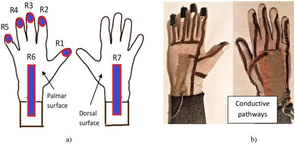
Figure 1 Smart glove design
