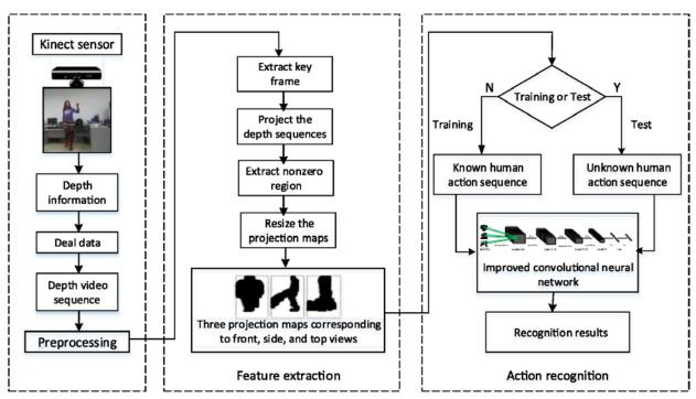
Figure 4 Typical motion recognition-shaping diagram (Lingin & Xiaolin, 2018)
