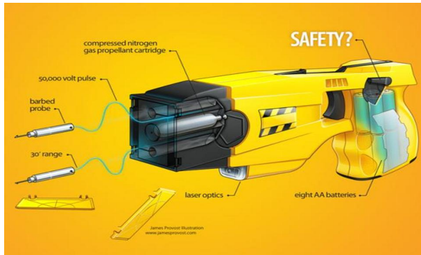
Figure 2. TASER X26 stun gun mechanism (Source: Products, webpage)
