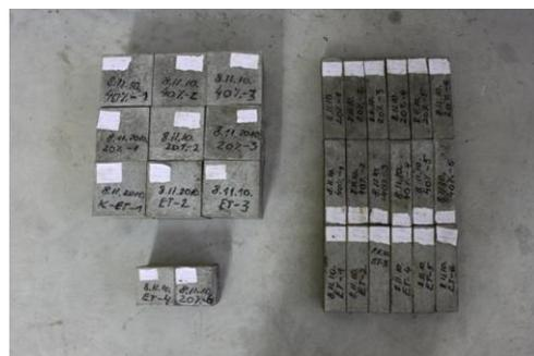
Fig. 1. Specimens containing lamp glass powder
