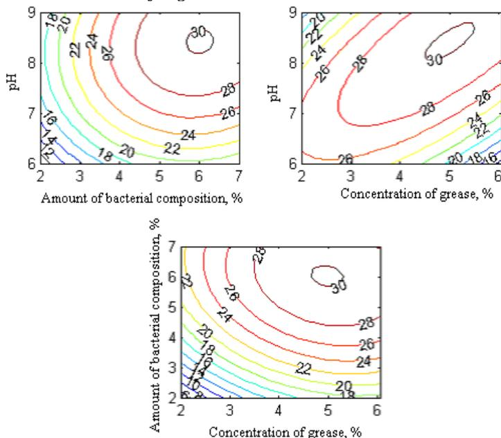
**Fig.2. Response surface of the amount of degraded grease depending on technological parameters**
