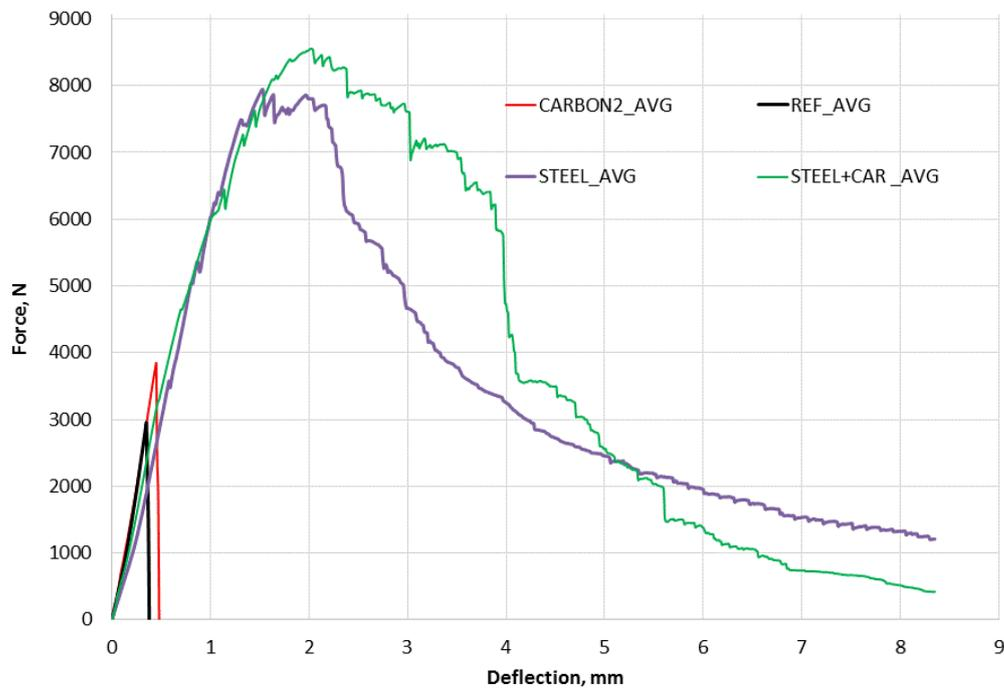
Fig. 3. Three-point bending force – deflection curves.
