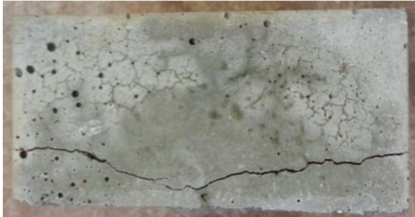
Fig. 6. The microcrack pattern of split UHSC sample cured at 200 °C for 4 h (HT3-200).
