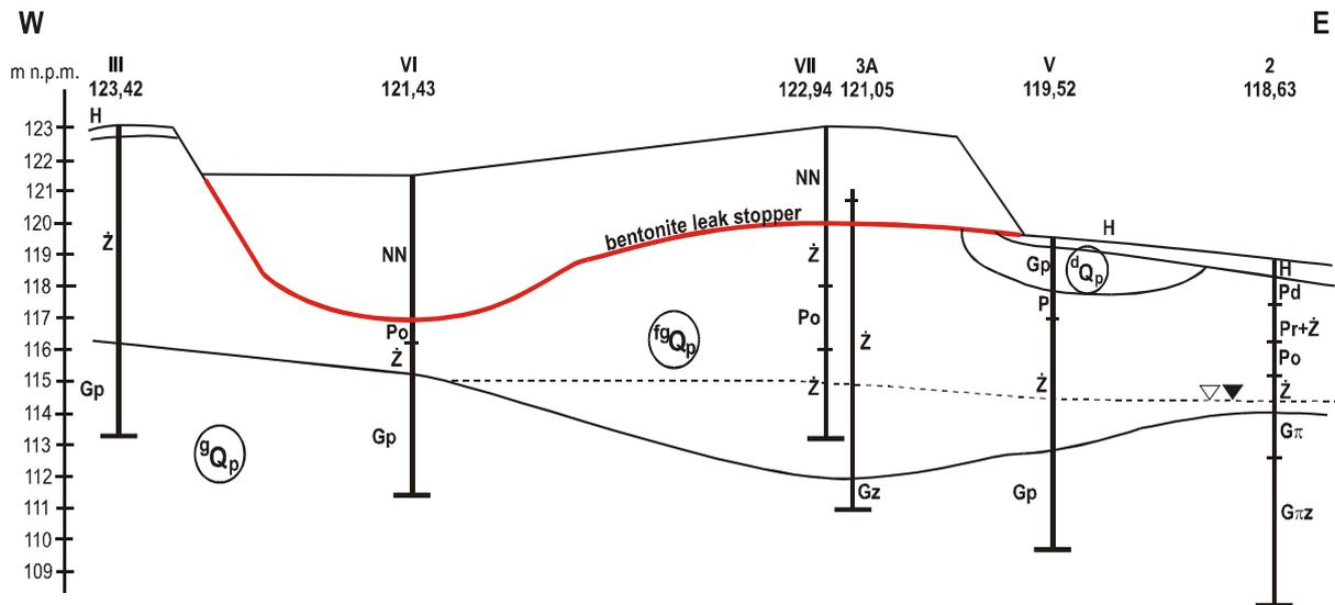
**Fig. 5. Geological cross-section C-C'**
