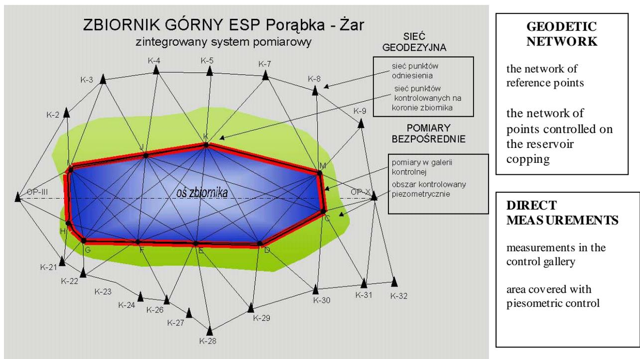
Fig. 6. The upper reservoir of the ESP Porąbka–Żar – a diagram of the integrated measurement
