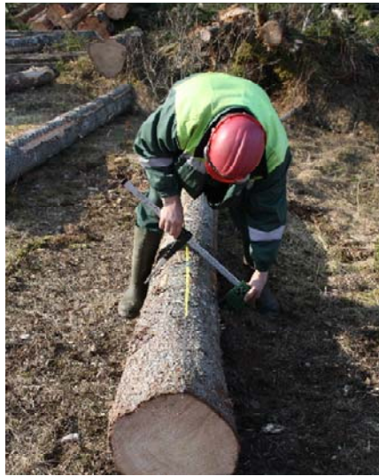
Fig. 8. The example of control of the harvester measuring system, where: the log N° 3 participated one of the 34 round wood assortments used in the process of control of harvester measuring system
