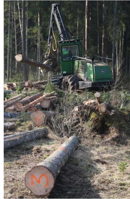
Fig. 8. The example of control of the harvester measuring system, where: the log N° 3 participated one of the 34 round wood assortments used in the process of control of harvester measuring system
