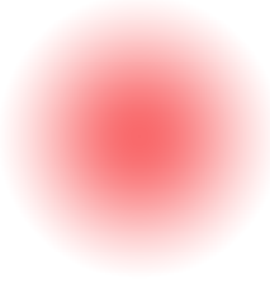
Fig. 2. Normal (Gaussian) distribution of energy within cross-section perpendicular to direction of laser pulse propagation
