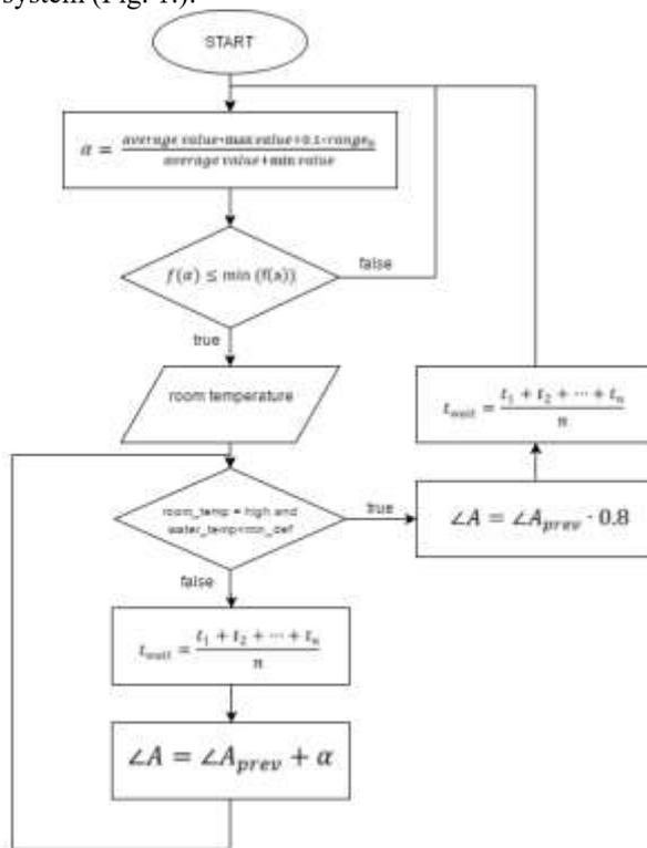
Fig. 1. Algorithm of the adaptive heating valve control system
