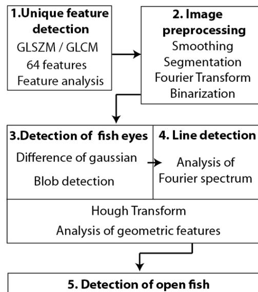
Fig. 2. Fish analysis system flowchart
